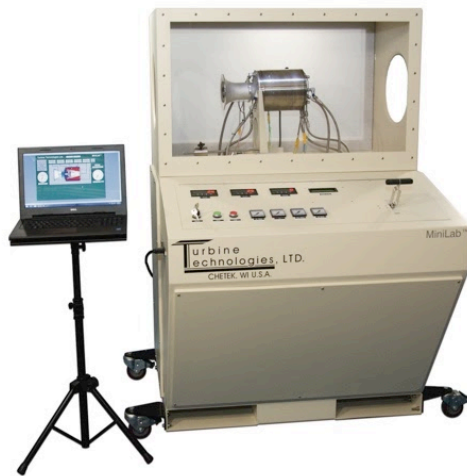
Figure 1 Commercial Example of Test Stand and Control System for WREN 75.
