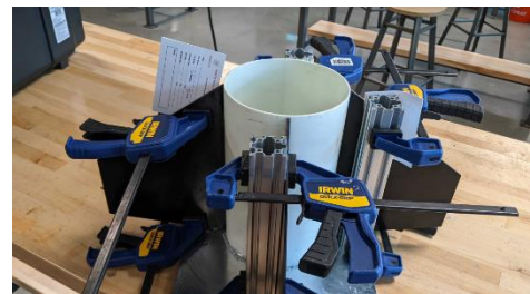
Figure 6. Fin alignment jig.
