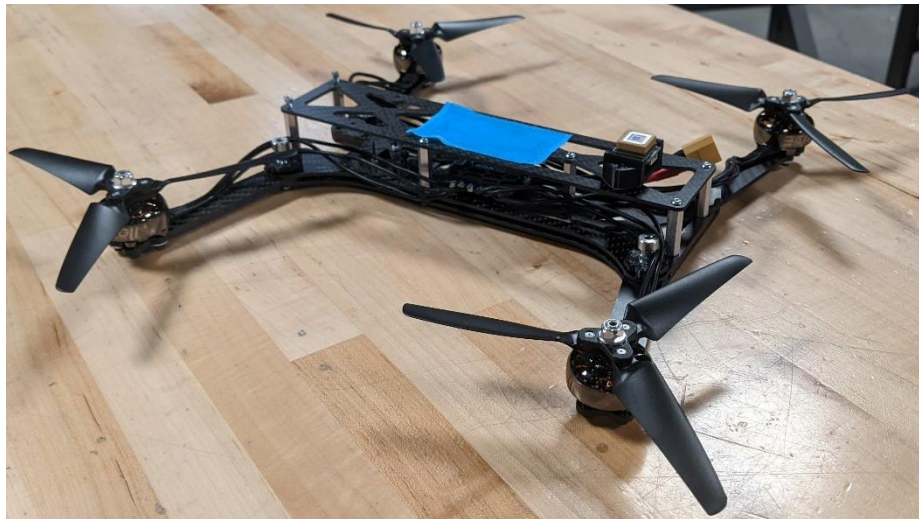
Figure 50. Quadcopter in the Unfolded Configuration.
