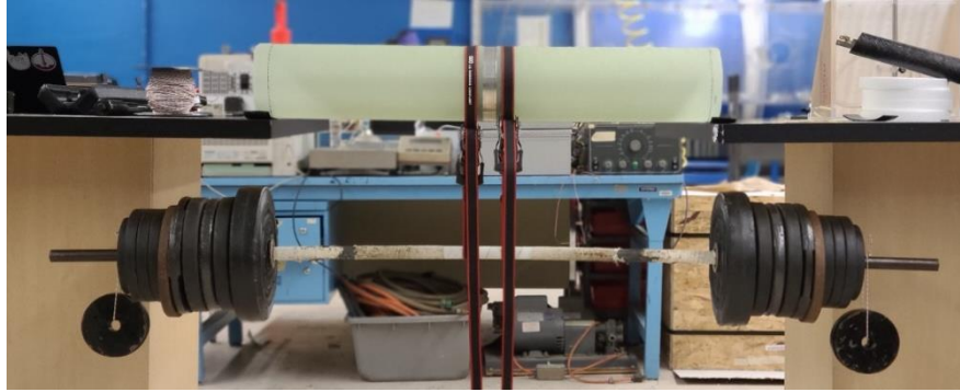
Figure 16. Coupling 3-point flexural test.
