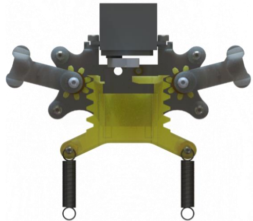
Figure 48. - Top view of payload arm deployment mechanism with gears and rack shown in yellow.
