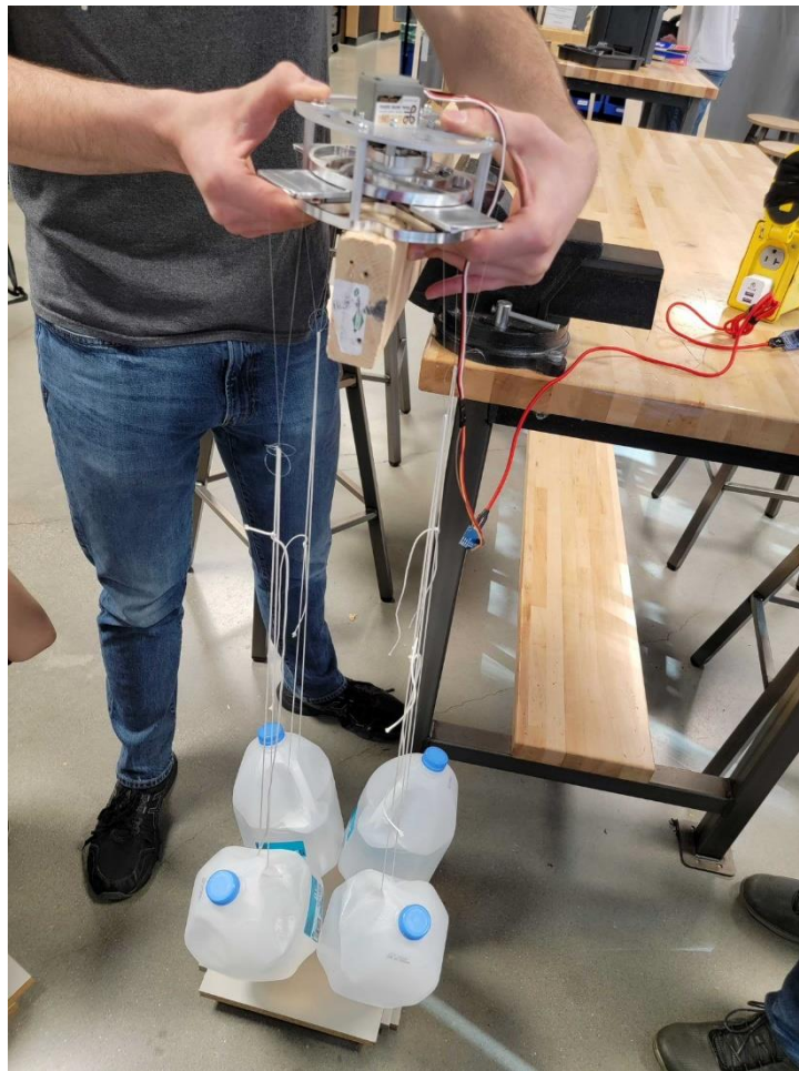
Figure 24. Airbrake actuation test.
