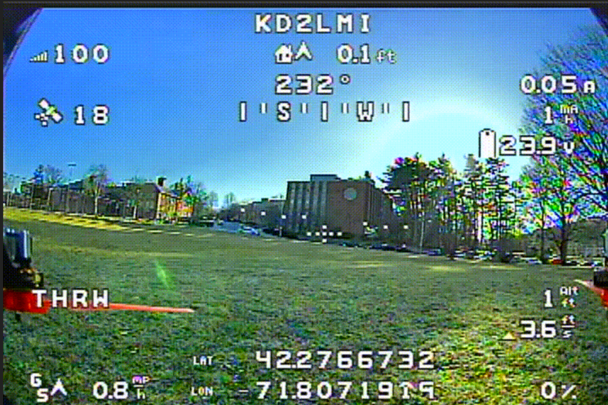
First Person View Signal with On Screen Display
