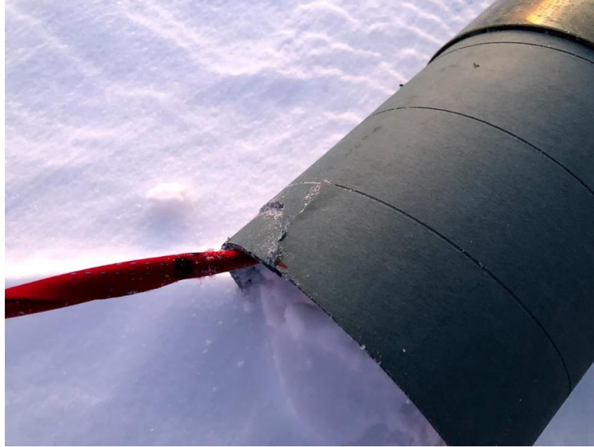
Figure 7-23 Upper Airframe Coupler Zippering
