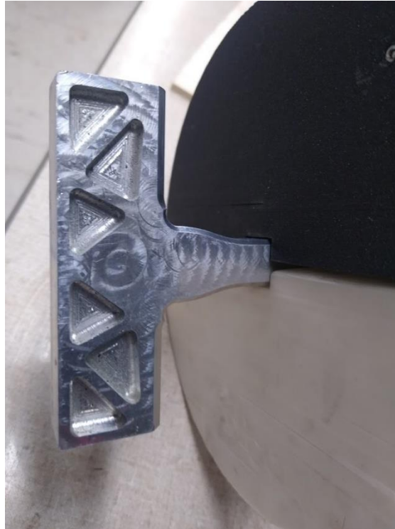
Figure 5-39 Mill marks on the final lightened spine. The chamfers on the upper surface help align it vertically during rotation.
