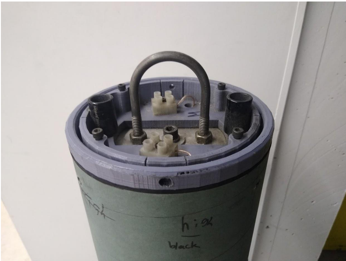
Figure 5-47 Ballast adapter print with ballast core tube removed, showing location of terminal blocks and ejection wells. The neoprene seal (black) is visible above the coupler tube
