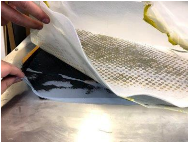
Figure 5-5 Fins being removed from vacuum bag.
