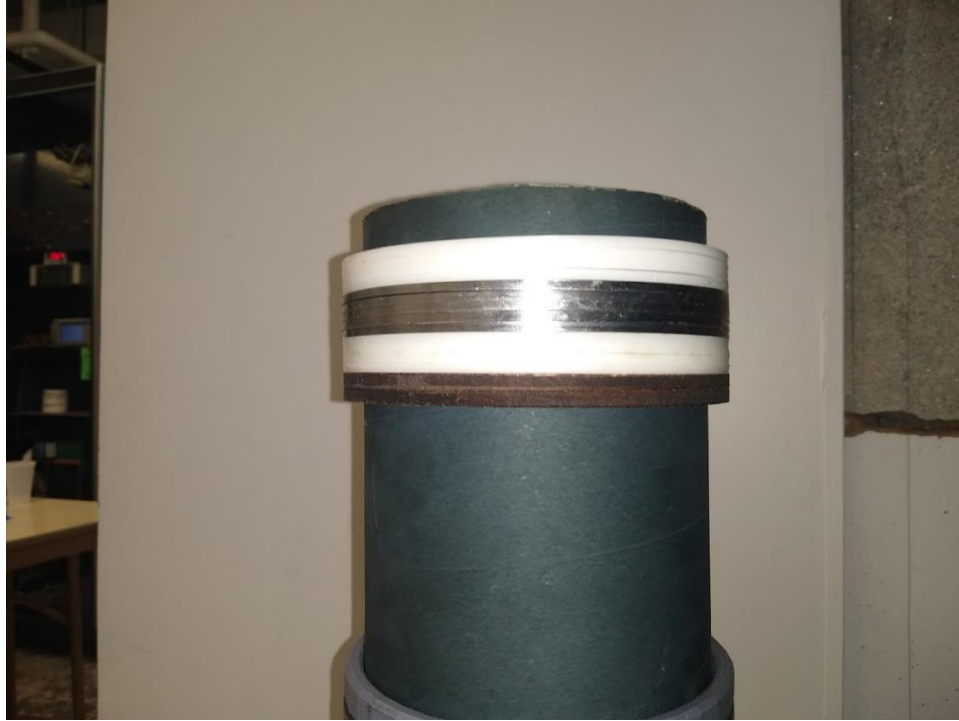
Figure 5-52 Ballast system with delrin and steel rings
