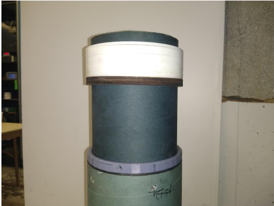
Figure 5-51 Ballast system with delrin rings.
