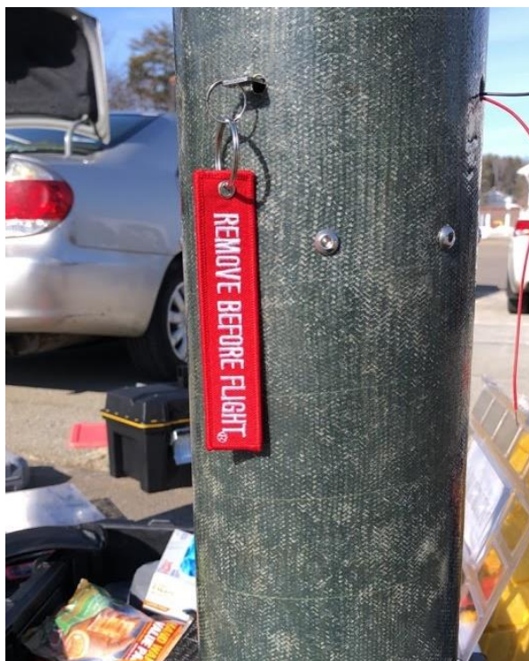
Figure 5-23 Key with remove before flight flag. Installation indicates that the electronics bay is in TEST mode. On the right: Power leads emerging from the external power port, in preparation for a ground test.
