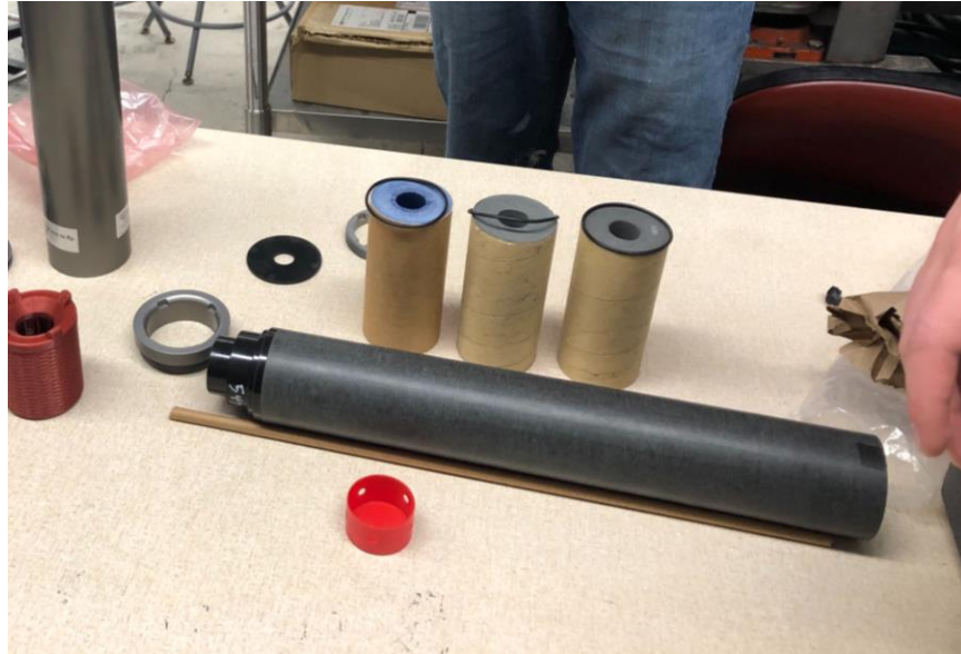
Figure 7-2: Motor Assembly and Grains
