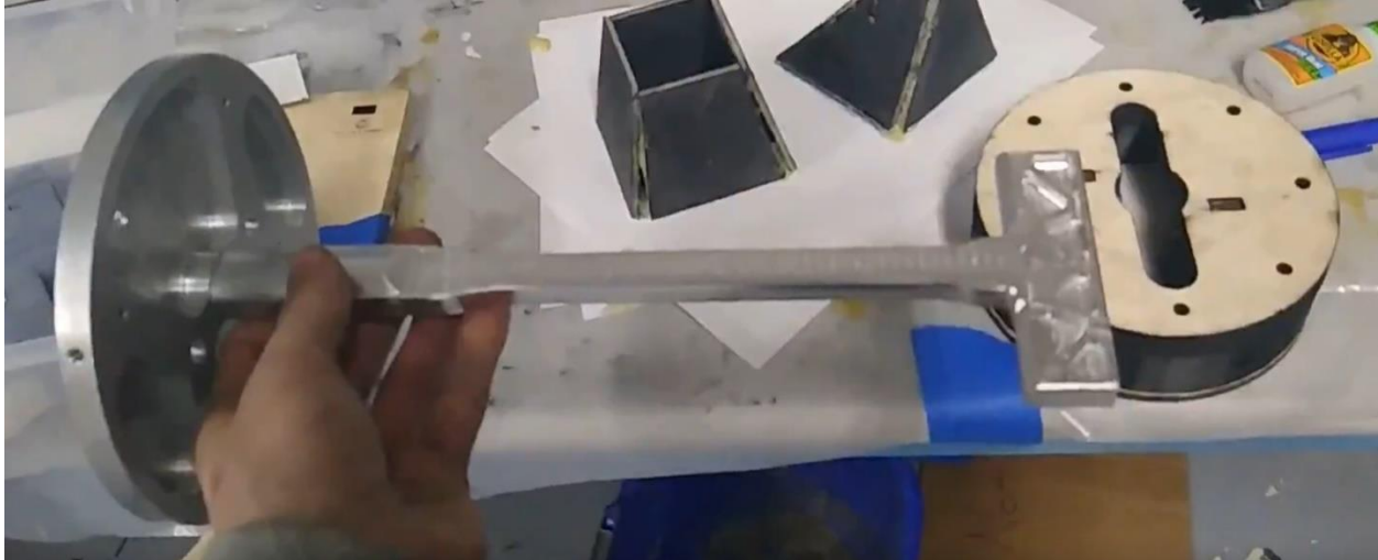
Figure 5-29 Forward bulkhead rigidly mounted to the aluminum spine
