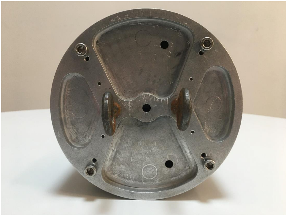
Figure 6-12 Payload retention bulkhead rear view
