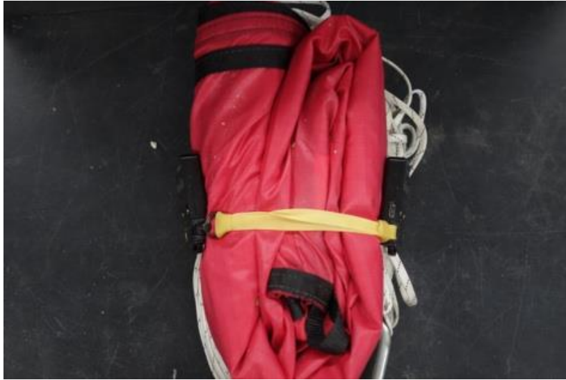
Figure 5-56 Jolly Logic Chute Release (side view). Jolly logics are connected in series for redundancy, such that only one needs to function correctly to release the parachute.
