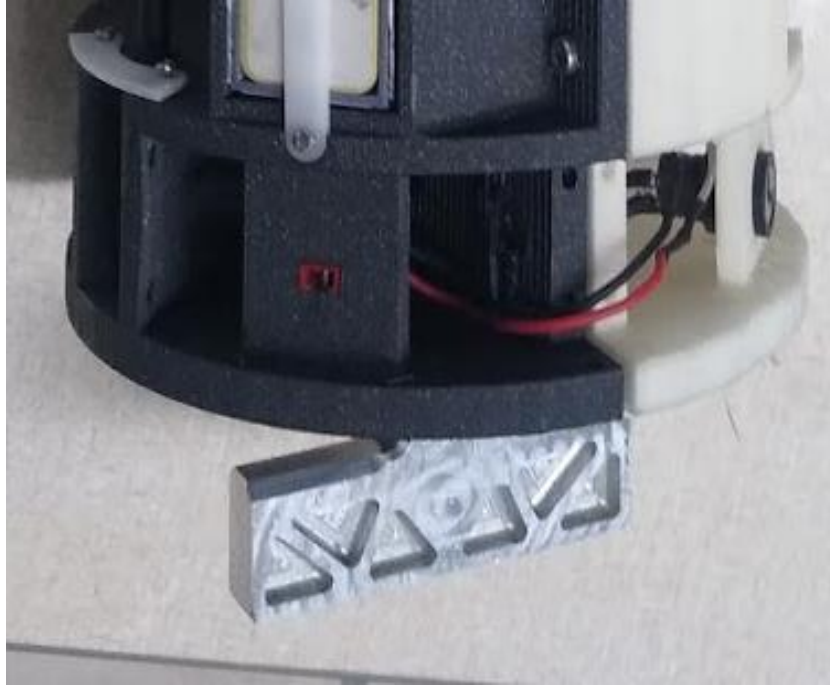
Figure 5-45 Band on which all externally accessed devices are mounted, to allow airflow up to Strattologgers
