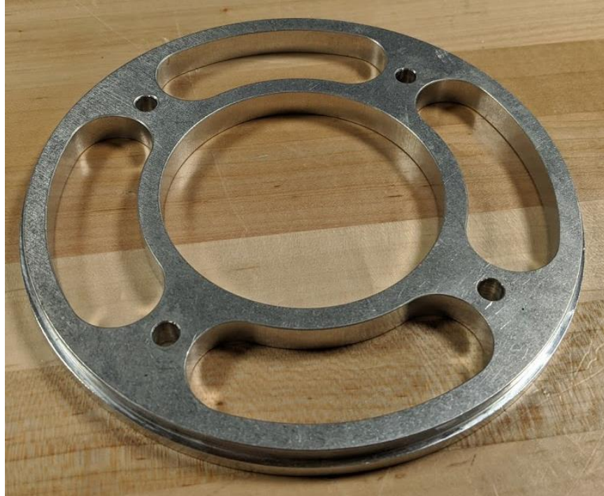
Figure 5-12: Completed Thrust Plate
