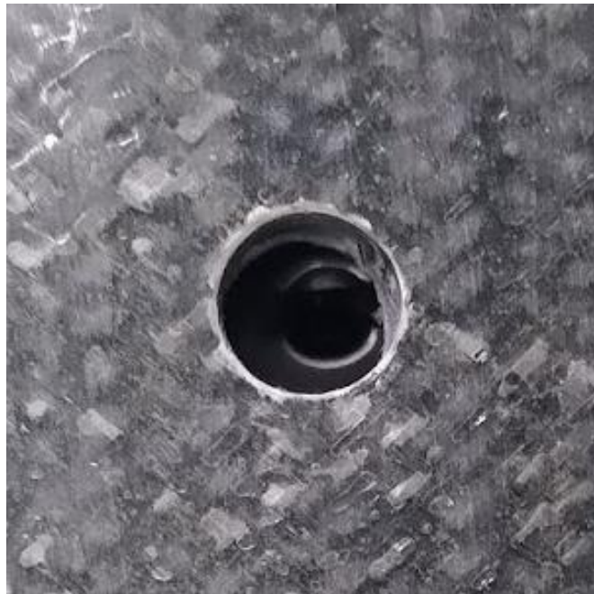
Figure 5-46 Alignment with key lock switch on fully assembled and installed sled with pressure sampling hole through airframe/coupler
