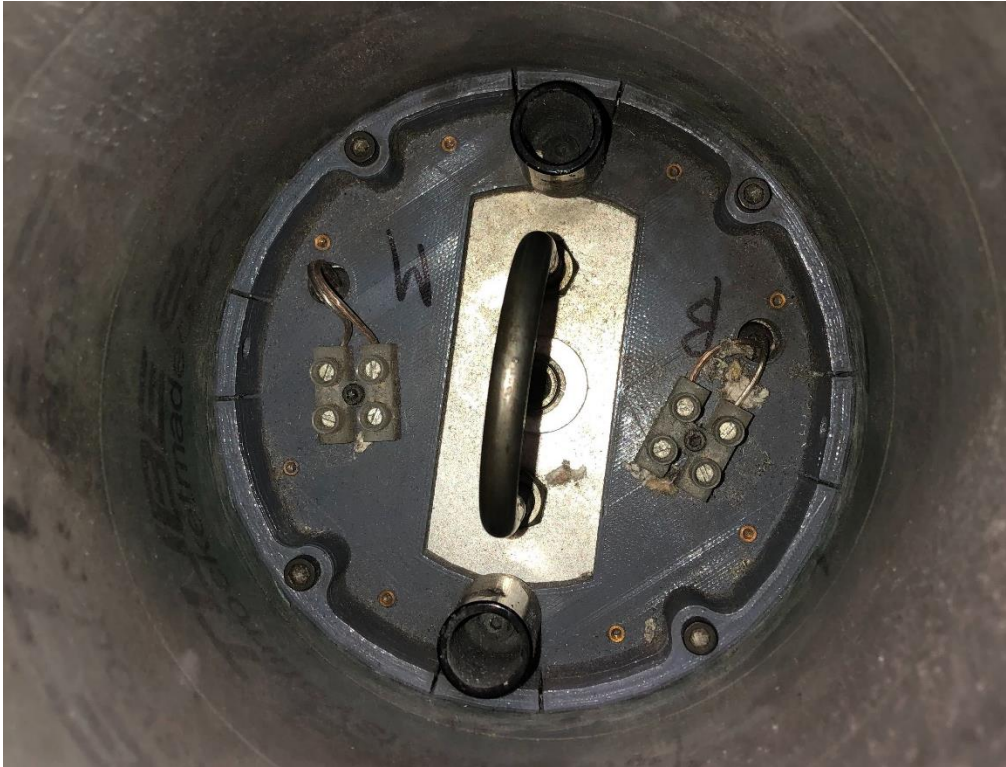
Figure 5-21 Forward bulkhead of the electronics bay, showing permanently connected wires routed through the bulkhead to the Strattologgers. Open ends of the terminal blocks (bottom) are used as a connection point for charge e-matches.
