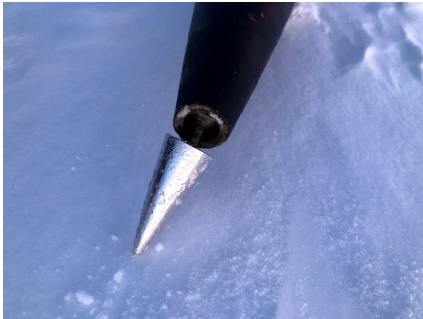
Figure 7-24 Nose Cone Tip Damage
