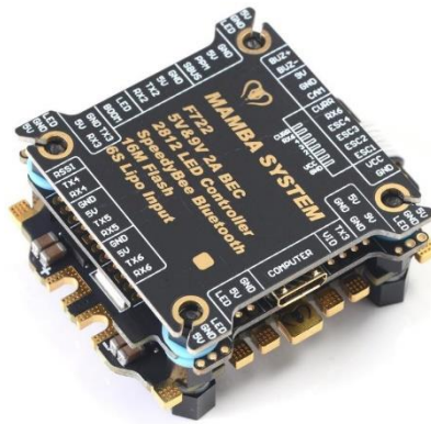
Figure 6.1.2.1 Diatone Mamba F722S Stack - 506 50A Dshot1200 6S ESC
