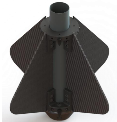
Figure 5.1.5.1 Showing Fin Can assembly
