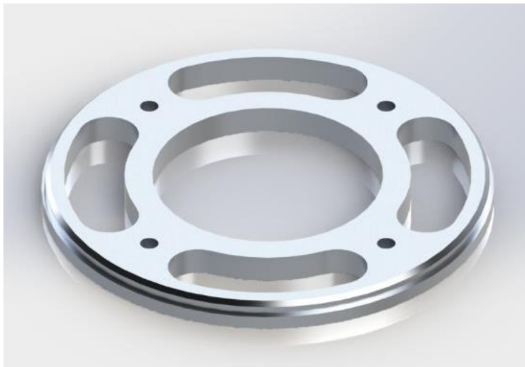
Figure 4.6.4 Diagram Showing the Back-Up Fin-Can Retention Design
