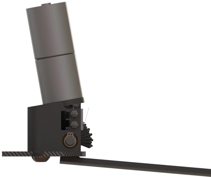
Figure 7-14 Side view of the motor mount with all components attached.
