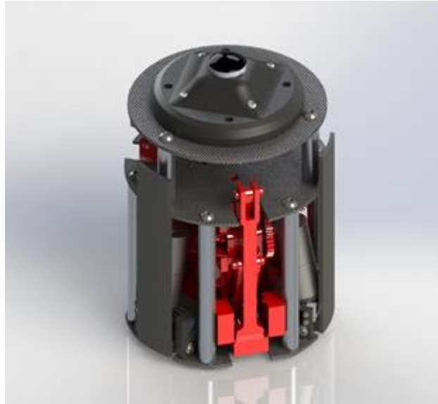
Figure 7-24 An isometric view of the payload top assembly. Stabilization modules in stowed configuration are highlighted in red.
