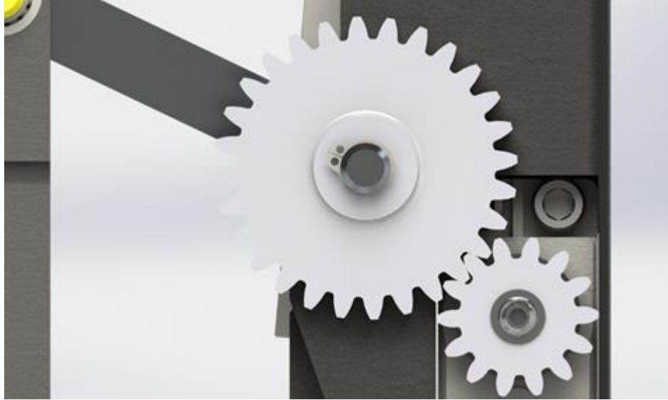
Figure 7-27 A right-hand view of the geartrain of the lift mechanism. Note the servo driving the 14-tooth servo on the right-hand side of the render
