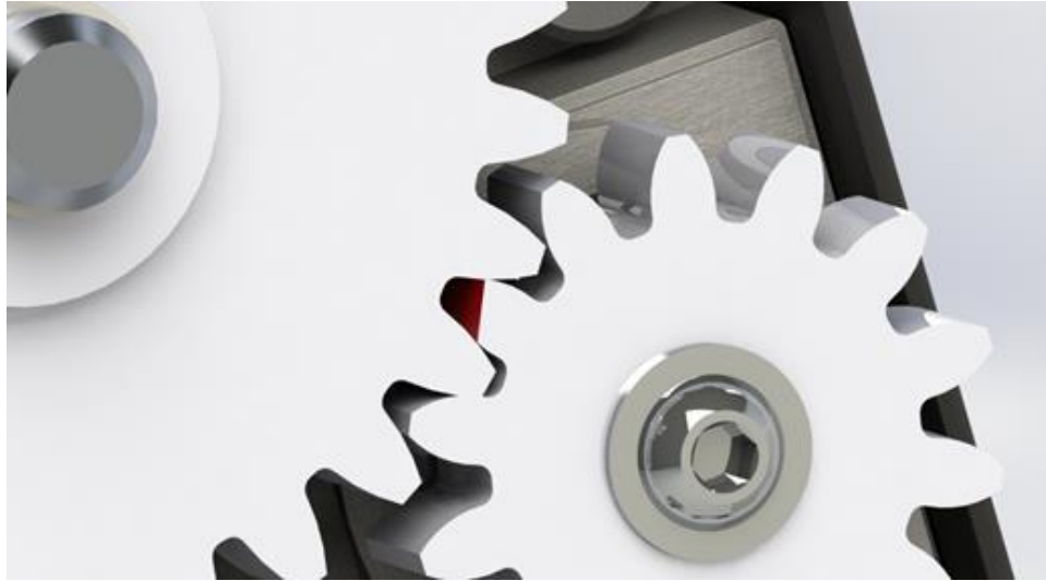
Figure 7-28 A skewed view of the stress plane of the driving gear. The section in red is offset 22.68 degrees from the plane tangent to both gears' pitch circles.
