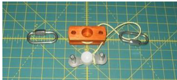
Figure 7.6 Fruity Chutes Tender Descender upon separation.
