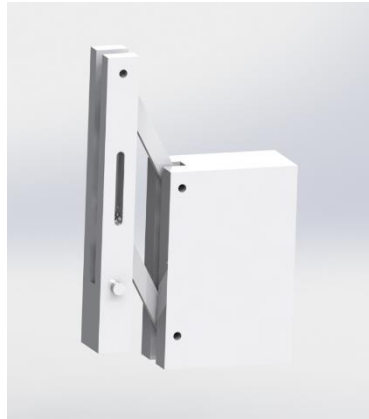
Figure 7.40 The arrested four bar linkage in its parallel phase of deployment
