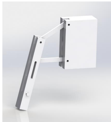
Figure 7.41 The arrested four bar linkage in its uneven phase of deployment
